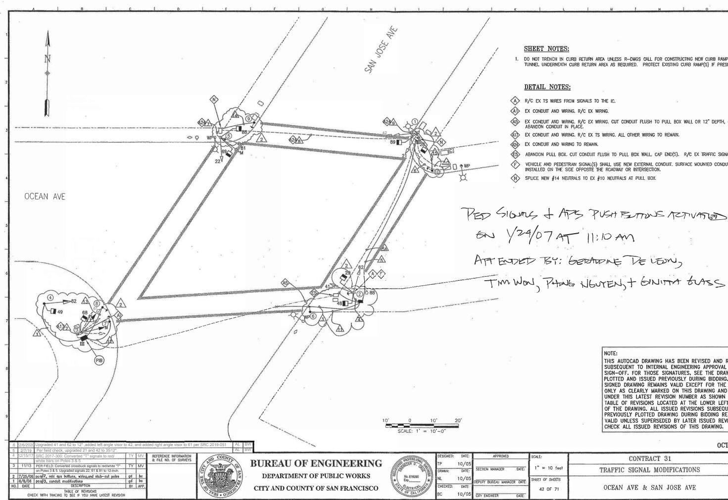
1. DO NOT TRENCH IN CURB RETURN AREA UNLESS R-DWGS CALL FOR CONSTRUCTING NEW CURB RAMPS. TUNNEL UNDERNEATH CURB RETURN AREA AS REQUIRED. PROTECT EXISTING CURB RAMP(S) IF PRESENT.
